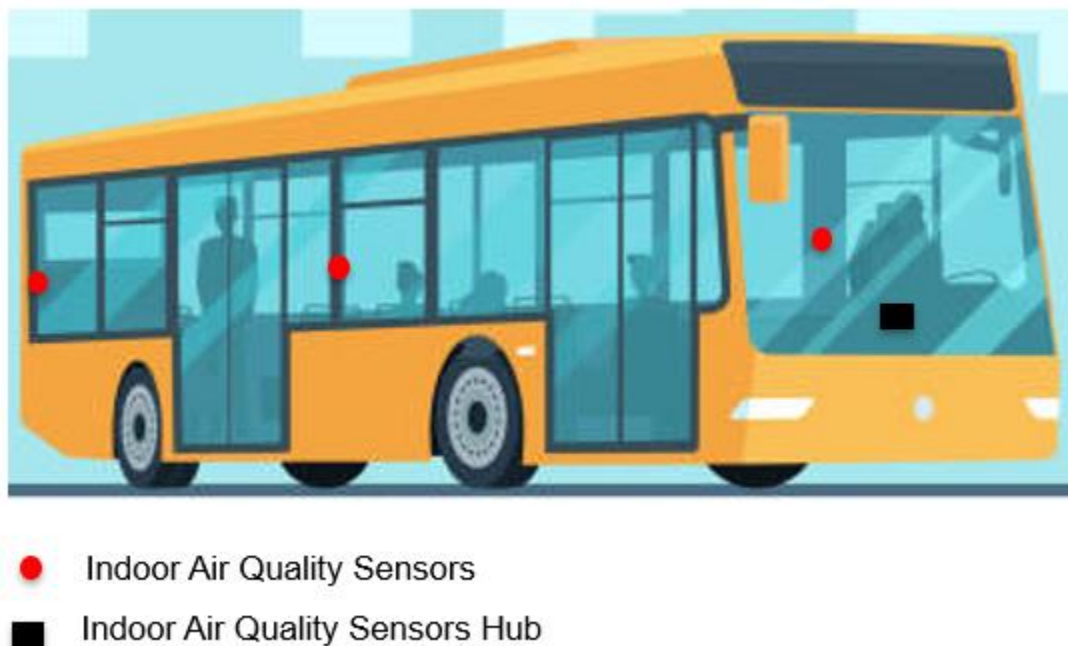
Figure 1: Example of a smart sensors installation in a bus cabin
